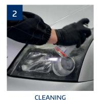
Mask the rear part of the headlight and clean the surface with SprayMax Silicone remover.
