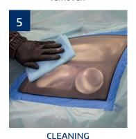
Clean surface between the sanding steps with Spay-Max Aqua-Silicone-Remover 680094.
